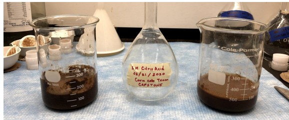
Figure 7-4: Citric acid saturation (Photo by: Kileigh Phillips)
