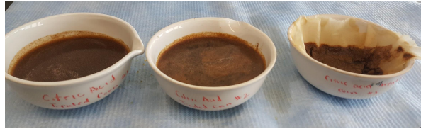
Figure 7-1: Dried citric acid treated corn cob (Photo by: Kaitlyn Tighe)
