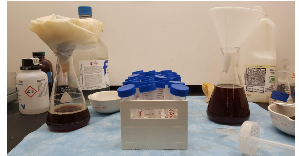
Figure 7-3: Corn cob and nitric acid solution being filtered in preparation for drying oven (Photo by: Kileigh Phillips)
