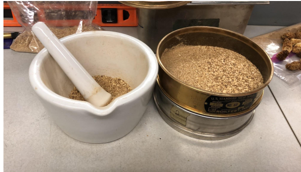
Figure 6-4: Mortar and pestle used to break down corn and 250 \mu\text{m} sieve (Photo by: Kaitlyn Tighe)
