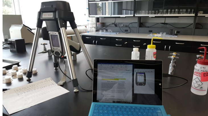
Figure 13-2: XRF device running final analysis of corn cob after 500 ppb Arsenic testing with citric acid and untreated corn (Photo by: Kaitlyn Tighe)
